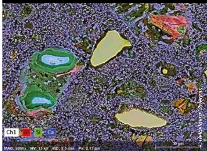
Figure 1: scanning electron microscope in the back scatter electron mode (cross-section across the compacted sample) with elemental map of the carbonated recycled concrete paste showing the main carbonation products
